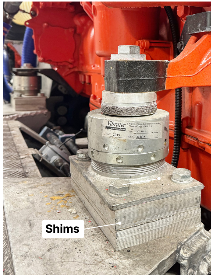
See an example of a marine engine setup with four of our VT41XX isolators (big brother to VT42XX). Here shims are used under the isolators to raise the engine position.
